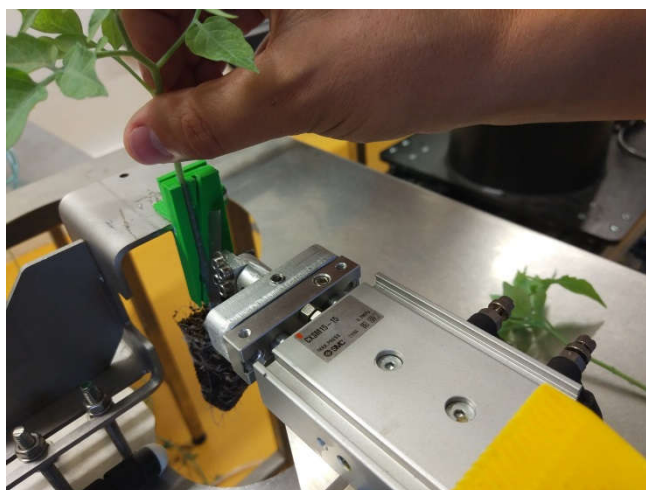
Figure 2. Cutting device. As can be seen, a fitting device is used to guarantee or ensure the verticality of seedling in the cutting process, beside a groove for insertion of the cutting blade. A specific fitting device for each cutting angle was developed. Once inserted, the seedling is dissectioned in two by a sharp blow of the sharp blade.
