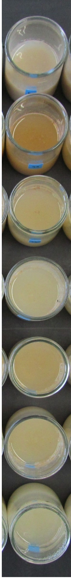
Figure S1: Color differences among extracts of the same soil sample treated with different H 2 O 2 solutions. From left to right, Wako, Showa, Kozakai, Kenei, Swan, Essential Oxygen, and AGA.
