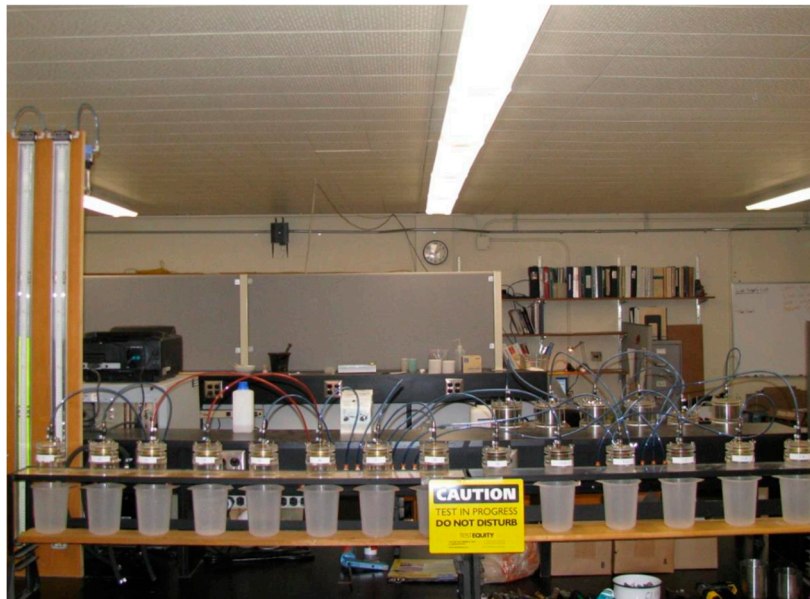
Figure 2. Setup of the Tempe cell experiment.
