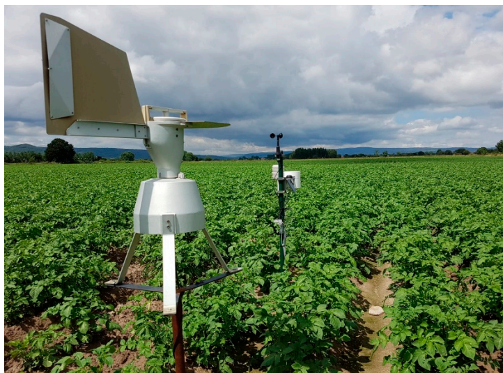
Figure 1. iMETOS ® 3.3. by Pessl Instruments weather station and Lanzoni VPSS 2000 volumetric sampler.
