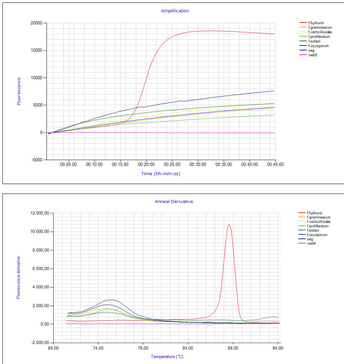
**Figure 5.** Validation of the analytical specificity of the LAMP reaction obtained with amplification of *F. fujikuroi* DNA (I1.3) compared to five other isolates of *Fusarium* belonging to the GFSC, *F. proliferatum* and *F. verticillioides*, and *F. graminearum*, *F. oxysporum* and *F. solani*.
