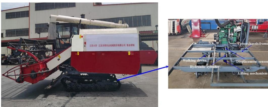
**Figure 12.** The prototype with the adaptive leveling system.
