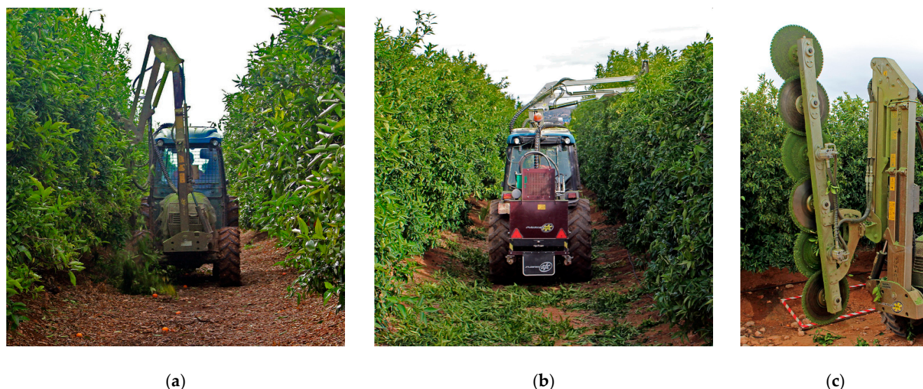
Figure 2. Tractor-mounted pruning machine used in the trials: (a) hedging cutting; (b) topping cutting; (c) articulated arm with six cutting discs.
