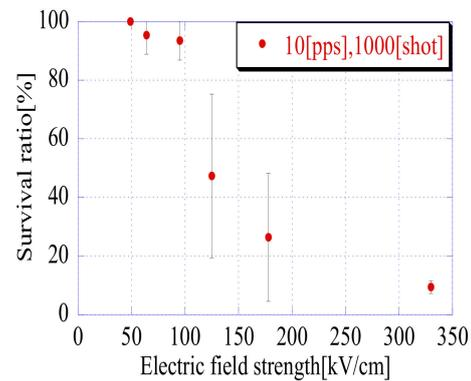
**Figure 20.** Survival ratio of *E. coli* for the electric field strength of the center of the bottom in the hollow in configuration (6).
