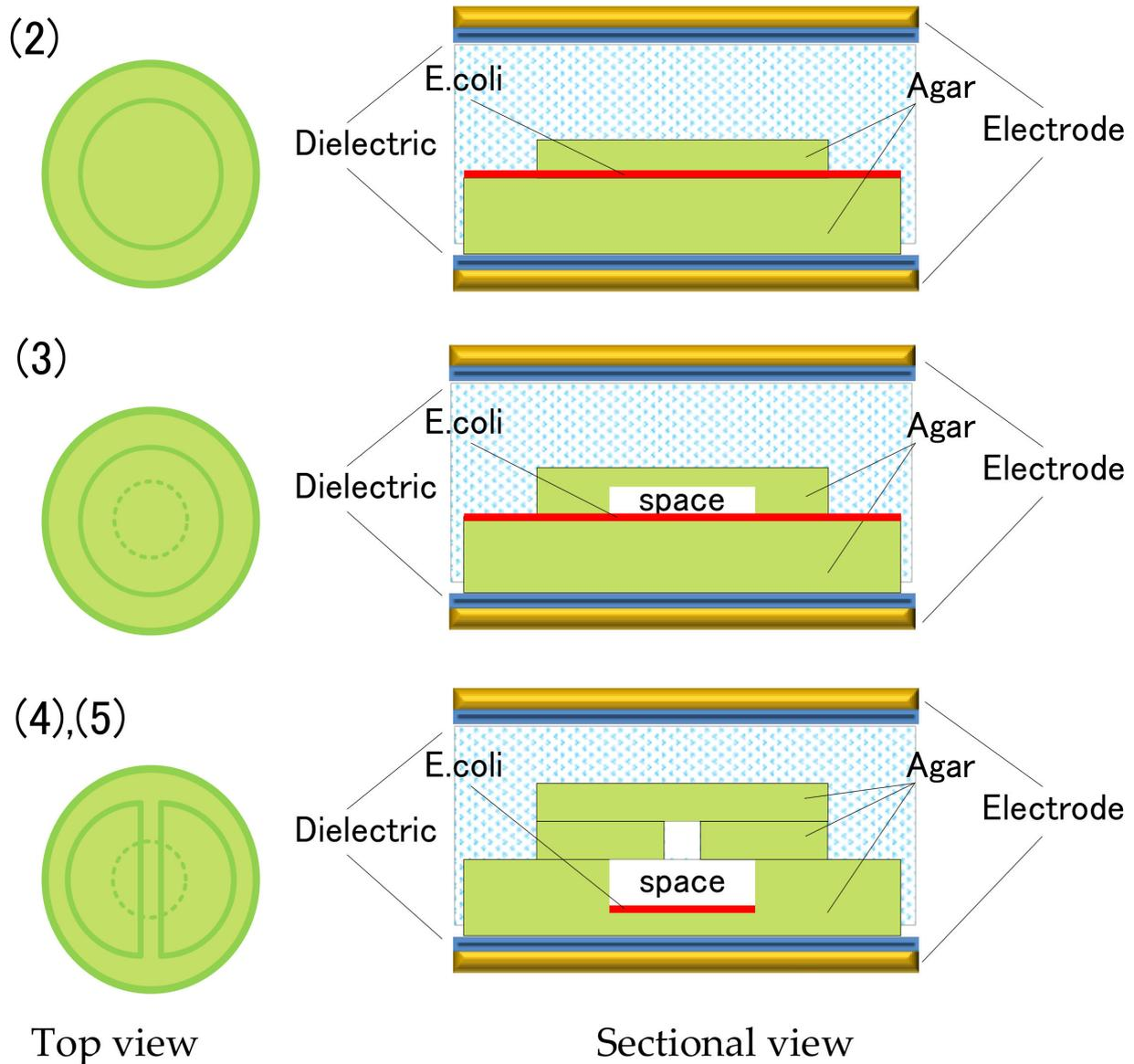
**Figure 8.** Agar medium configurations and positions of *E. coli*.
