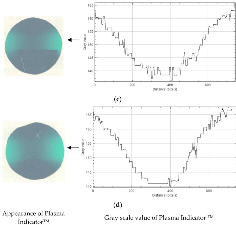
**Figure 13.** Color change of Plasma Indicator™ and gray scale value for each pulse number. (a) 500 shots; (b) 1000 shots; (c) 5000 shots; (d) 10,000 shots.
