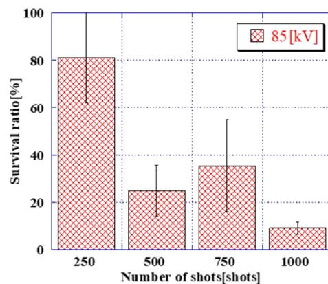
**Figure 17.** The survival ratios of *E. coli* after applying plasma of each pulse number in configuration (6) (depth of hollow: 0.5 mm).
