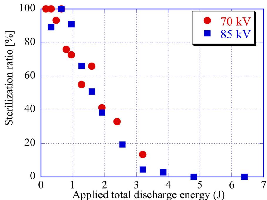
**Figure 7.** Survival ratios of *E. coli* on the surface of agar medium in configuration (1) for applied total discharge energy.
