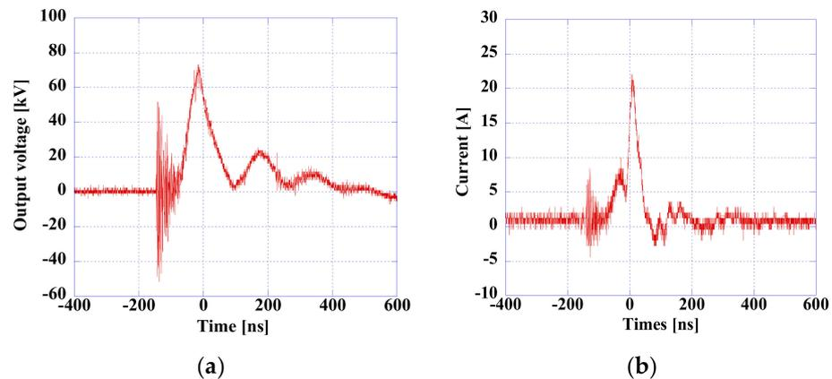
**Figure 4.** Typical applied waveforms to the petri dish (charging voltage: 10.5 kV); (a) voltage waveform; (b) current waveform.
