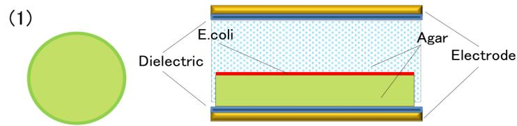
**Figure 5.** Agar medium configuration (1) and position of *E. coli*.
