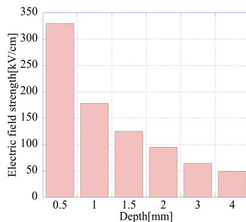
Figure 19. Electric field strength of the center of the bottom in the hollow calculated by the simulation for each depth of hollow in configuration (6).
