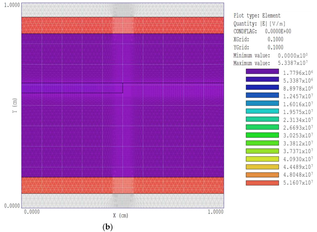
**Figure 16.** Simulation result of electric field distribution for configuration (6). (a) With polyimide film; (b) without polyimide film.
