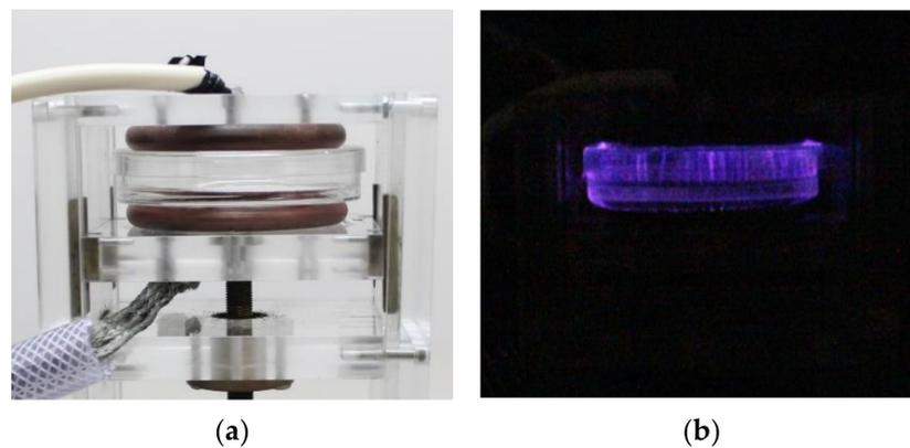
**Figure 3.** The electrode for applying pluses; (a) appearance of the electrode; (b) appearance of the generated plasma.
