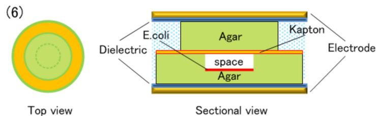
**Figure 15.** Agar medium configuration (6) with the polyimide film and positions of *E. coli*.
