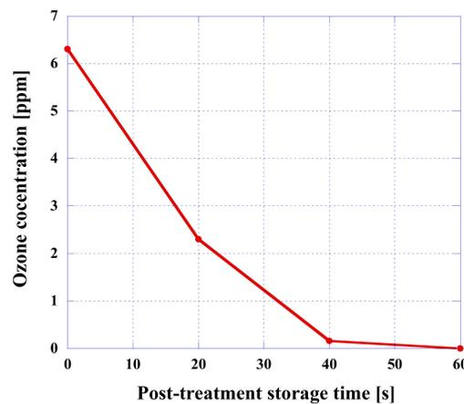
**Figure 14.** Ozone concentration in petri dish for elapsed time after pulse application. (Agar medium configuration (1); applied pulse voltage: 70 kV; applied pulse number: 100 shots).
