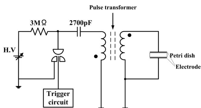
Figure 2. Pulsed plasma generating circuit.
