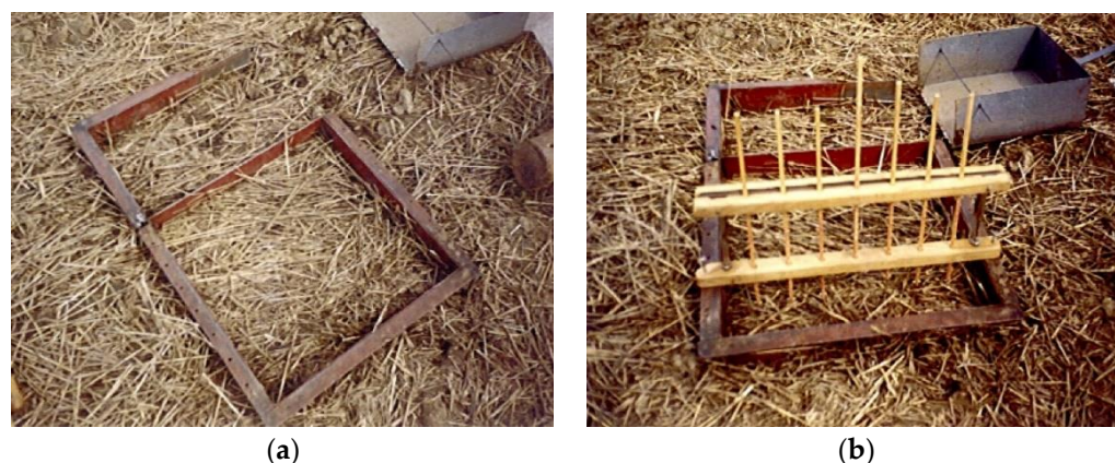
Figure 1. Steel frames, pressed to the soil (a); the measurement of seedbed surface roughness using a K. Trečiokas profilometer (b). The profilometer has seven rulers that measure the distance from the frame and seedbed surface. The measurements were performed at seven frame spots, resulting in a total of 49 seedbed surface measurements. These data were used for evaluation of seedbed surface and bottom roughness and sowing depth.
