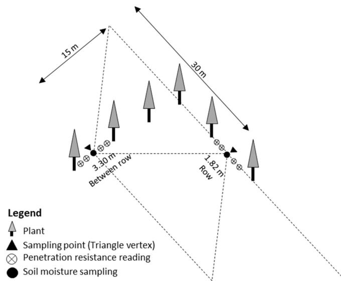
**Figure 2.** Sampling scheme for penetration resistance (PR) and soil moisture in coppicing and stand renewed with different straw levels 100, 50 and 0% areas, both preceded by eucalyptus harvest with Harvester + Forwarder (HF) and Feller + Skidder (FS). Sampling points are defined by the vertices of isosceles triangles (15 m of height and 30 m of base).
