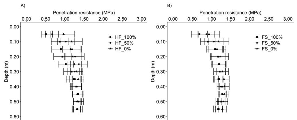
**Figure 4.** Soil penetration resistance (PR) up to 0.60 m depth in eucalypt cultivation areas under stand renewal with different straw levels (100, 50, and 0%) and harvested with (A) harvester + forwarder (HF) and (B) feller + skidder (FS) systems. Bars refer to the confidence interval (90%) of the average ( $n = 22$ ).
