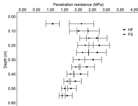
**Figure 3.** Soil penetration resistance (PR) up to 0.60 m depth in eucalypt cultivation areas under coppicing harvested with harvester + forwarder (HF) and feller + skidder (FS) systems. Bars refer to the confidence interval (90%) of the average ( $n = 22$ ).
