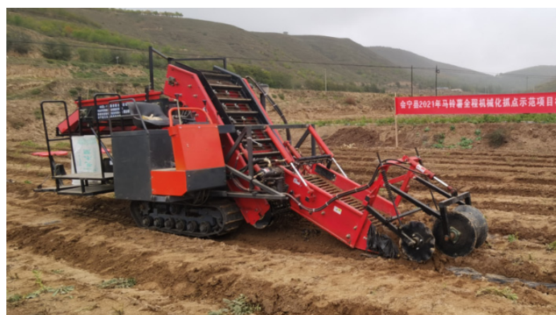
Figure 18. Field trial of the small-scale self-propelled potato combine harvester.
