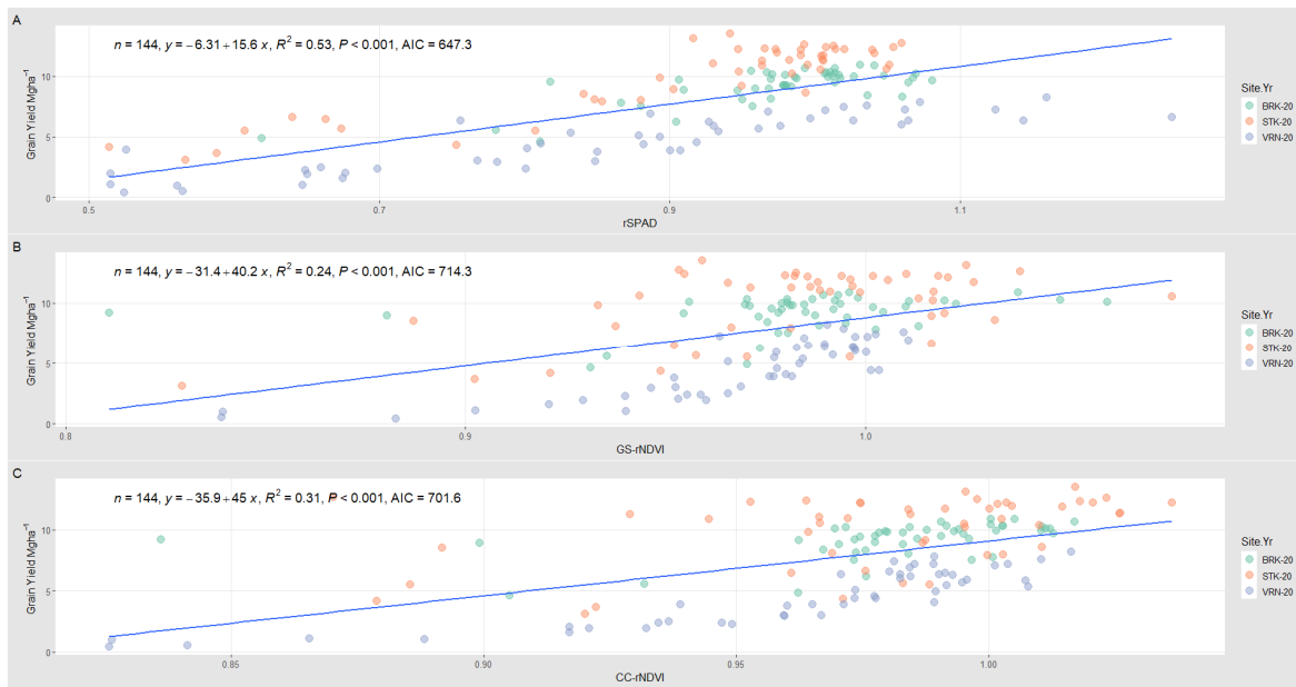
Figure 2. Sensor comparison between the relative VI values for the SPAD (A), GreenSeeker (B), and Crop Circle sensors (C) at the VT stage. The population for each equation is represented by n, the equation is represented by y, the coefficient of determination is represented by R 2 , the p-value by P, and the Akaike Information Criterion by AIC.
