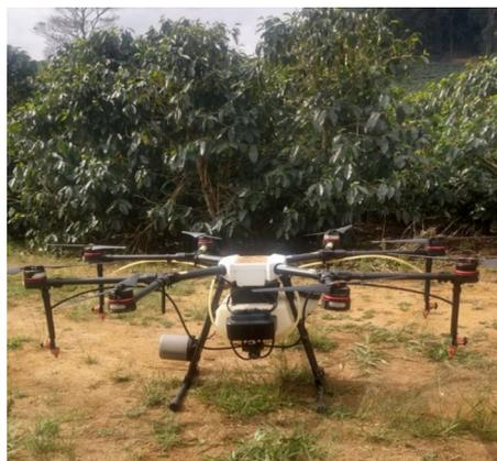
Figure 1. Multirotor unmanned aerial vehicle used for spraying in the experiment.
