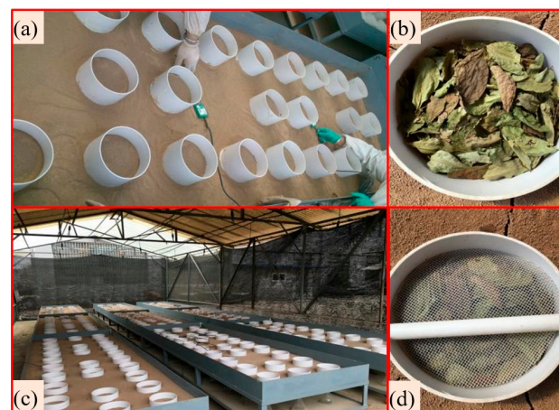
Figure A1. Experimental setups and PVC decomposition tubes used in this study. (a) A technician embeds probes that use time-domain reflectometry to measure soil moisture and temperature. (c) Screened, native soil beds under shade and with sunken experimental tubes. (b,d) Sunken tubes containing (b) uncovered leaf litter and (d) leaf litter covered by nylon netting.
