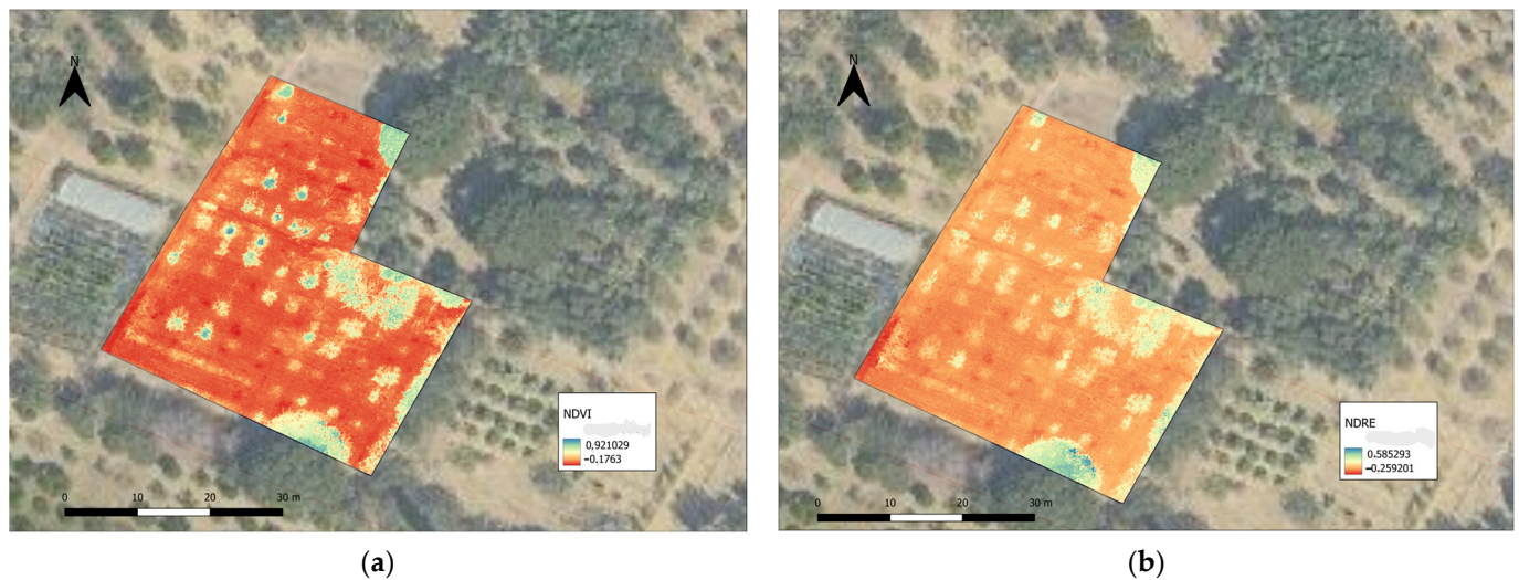
Figure 5. Map of the area of the study with the calculated NDVI (a) and NDRE (b) for the flight of 24 September 2021. Similarly, the same maps were generated for all of the flights. On this date, NDVI values ranged from -0.17 to 0.92 while NDRE values ranged from -0.25 to 0.58 .
