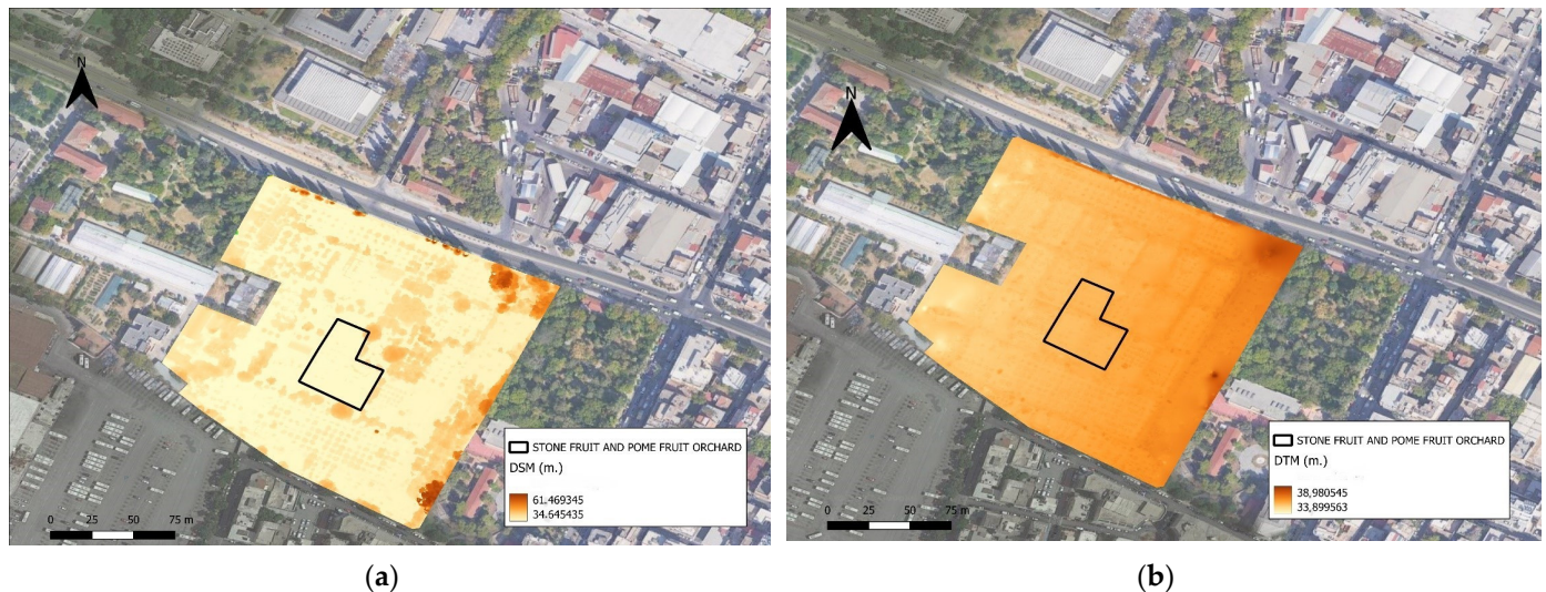
Figure 4. (a) Digital surface model (DSM) and (b) digital terrain model (DTM) of the orchard of Agricultural University of Athens. The stone and pome fruit orchards can be seen with a black border.
