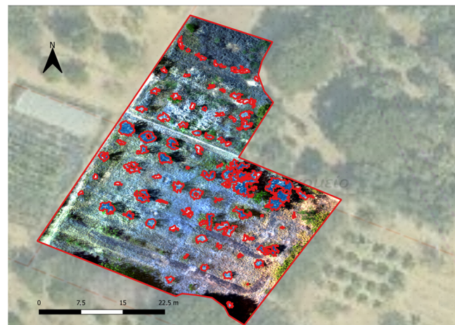
Figure 6. Digitization map of the trees in the orchard of the study for the flight of 28 May 2021, having calculated mean NDVI values for every tree. The same method was used in all of the flight dates so as to calculate the mean NDVI and mean NDRE values, as well as the area of the trees.
