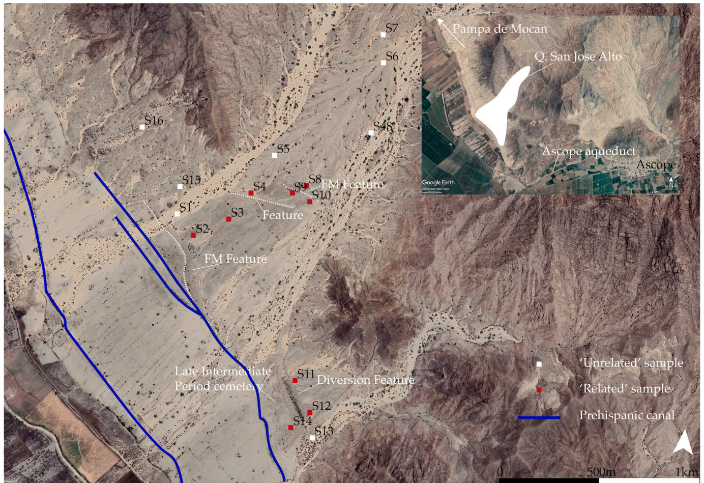
Figure 3. Quebrada San Jose. Floodwater management (FM) features and diversion feature labeled. Soil sample locations, and their ‘relatedness’ to the features also labeled. Google Earth Pro (2019) UTM 17 M 703374.9 E; 9148571.46 S.
