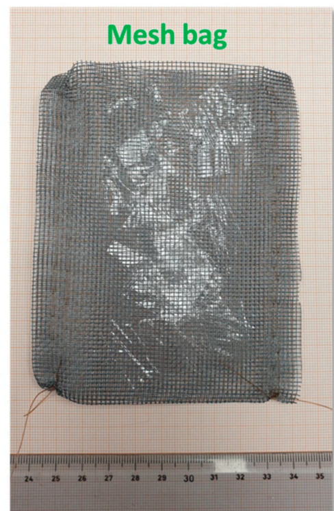
Figure 1. Preparation of biopolymer samples for anaerobic digestion: PLA films cut into 2.5 \times 2.5 \text{ cm} squares and enclosed in mesh bags for reactor incubation.
