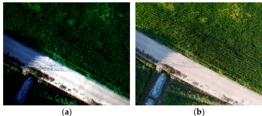
Figure 4. Multispectral band image registration and fusion results. (a) RGB image after registration; (b) reference image.
