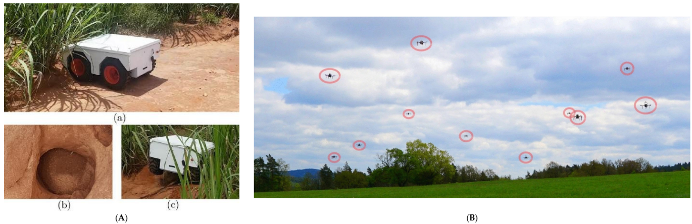
Figure 4. Application of swarm coordination technology in crop health monitoring. (A) Field tests of monitoring tasks in sugarcane fields. (a) robot entering the tunnel; (b) uneven terrain and big crevices; (c) robot passing over crevice, the structure is tilted and struggles to overcome the valley. (reproduced from [57]; CC BY 4.0) (B) Eleven unmanned aerial vehicles were used for on-site verification monitoring and target detection (reproduced from [59]; CC BY 4.0).
