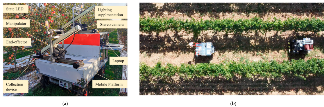
Figure 10. Applications of swarm control in orchard harvesting. (a) Structural diagram of the harvesting robot test platform based on dual manipulator (reproduced from [96]; CC BY 4.0). (b) Two robots within a vineyard row while coordinating their motions (reproduced from [98]; CC BY 4.0).
