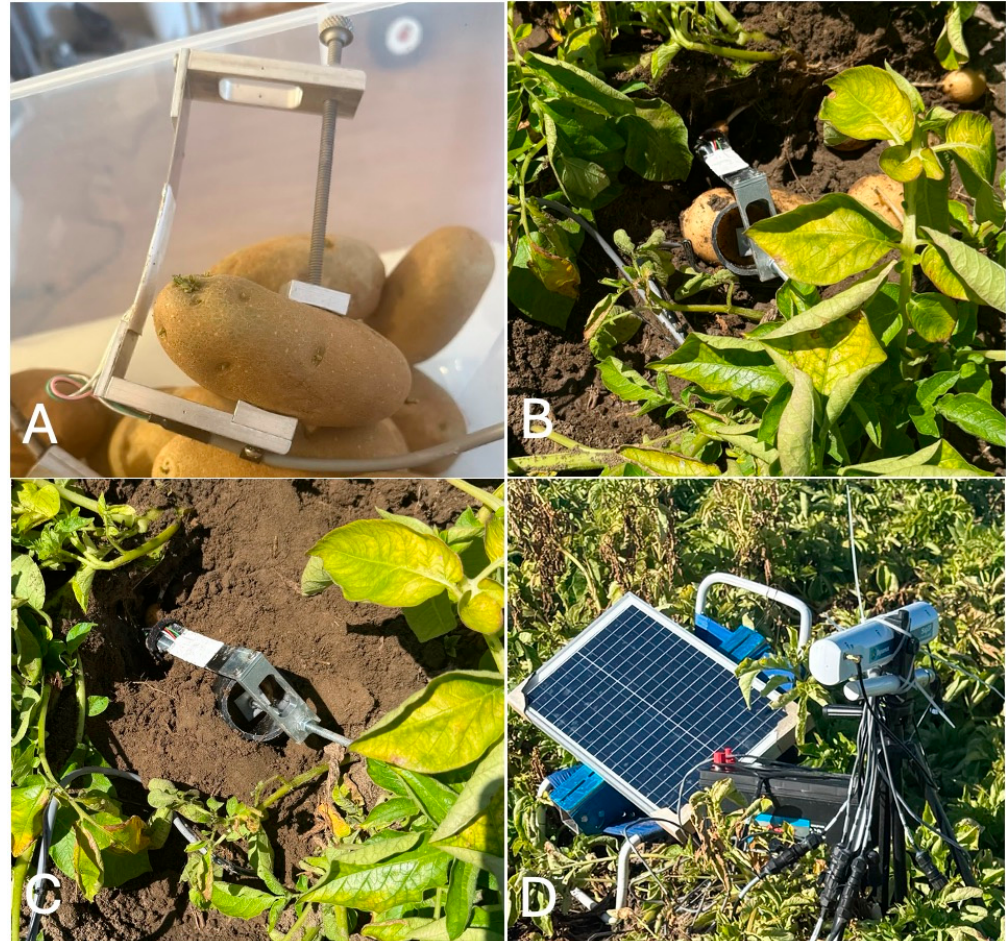
Figure 1. Tuber sensor and field implementation. (A) The strain gauge C-clamp [6] model DEX100 (Dynamax Inc., Houston, TX, USA) on a potato tuber. (B) The sensor was placed on the cleaned upper surface of the tuber. The metal anvil contacts the cleaned tuber and is inserted through an approximately 3 cm long black plastic pipe, flush with the tuber surface, pointing north. (C) The sensor on the buried tuber, except where the soil was blocked by the black plastic pipe. The square metal anvil is touching the potato inside the pipe, as shown in Figure 1A, and is positioned to measure the height dimension. (D) The equipment (Dynamax, Inc.) set up on 9 July included a solar panel, a 12-volt deep-cycle battery, an air temperature sensor inside the white acrylonitrile butadiene styrene (ABS) plastic data logger housing, and a data logger with a transmitter mounted on a tripod.
