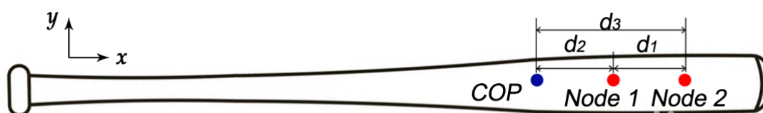
Figure 2. Distances between node 1, node 2 and the COP on the barrel of a baseball bat.
