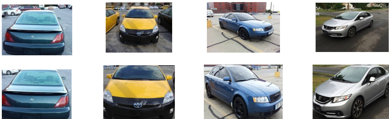
Figure 5. Sample images showing how noisy backgrounds are removed to improve training efficiency. The first row shows images with noisy background where other vehicles can be seen, oftentimes of different colors. The second shows the corresponding cropped images with background noise removed.
