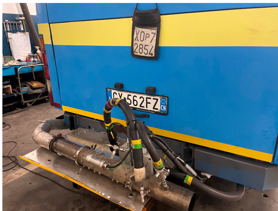
Figure 2. PEMS probe system connected to the exhaust of the Euro III bus used for road tests. The instruments were placed inside the bus (see Figure 3).
