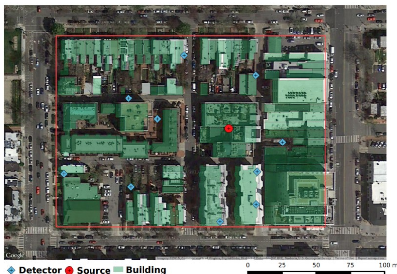
Figure 1. Satellite image of problem domain with model geometry overlaid (Imagery ©2016 Commonwealth of Virginia, DigitalGlobe, District of Columbia (DC GIS), Sanborn, U.S. Geological Survey, Map data ©2016 Google). The figure marks indicate possible detector and source locations.
