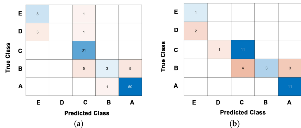
Figure 10. kNN classifier (run 21): confusion matrices relevant to the (a) training and (b) testing datasets.
