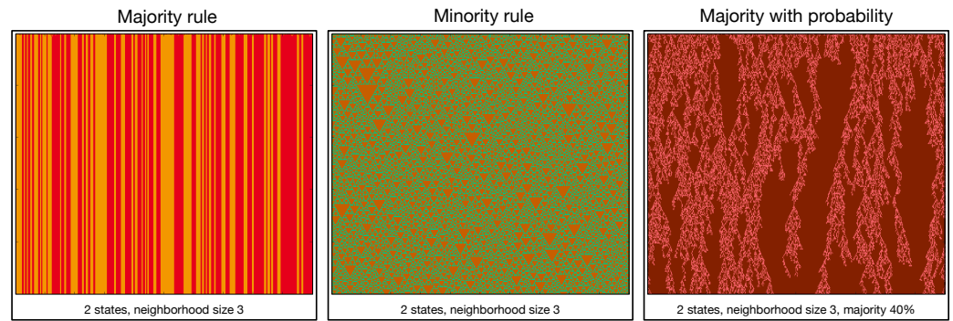
Figure 1. Examples of cellular automata with two states and a neighborhood size of 3, applying majority, minority, and majority with probability evolution rules.
