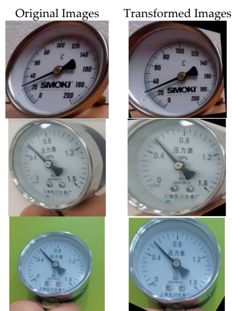
Figure 2. Comparison of pointer instrument dials before and after perspective transformation.
