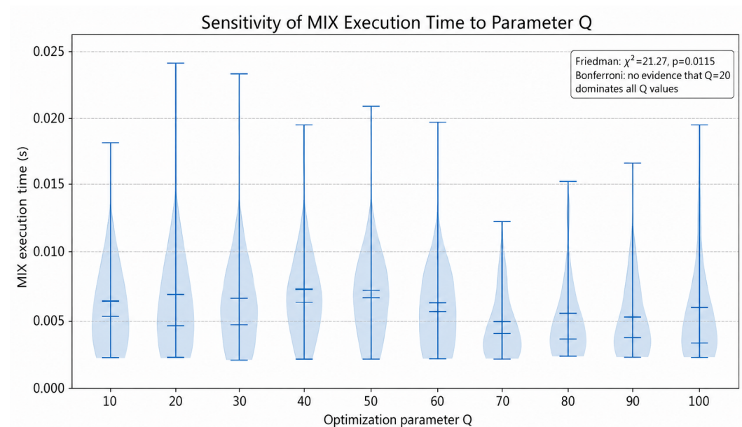
Figure 5. Sensitivity of SAT deterministic inference time to the \text{mix}(Q) parameter across the 25 benchmark networks. Violin plots show the distribution of mean execution times per dataset for each Q configuration ( Q = 10, \dots, 100 ). The inset reports the Friedman repeated-measures test result ( \chi^2 = 21.27 , p = 0.0115 ), confirming that Q significantly influences execution time. However, Bonferroni-corrected pairwise comparisons provide no evidence that any single configuration is statistically dominant over all others. The y-axis lower bound is fixed at 0s by definition. Low Q values (10–20) tend to produce lower medians and can serve as practical defaults, but no universally optimal configuration exists across all evaluated network structures.
