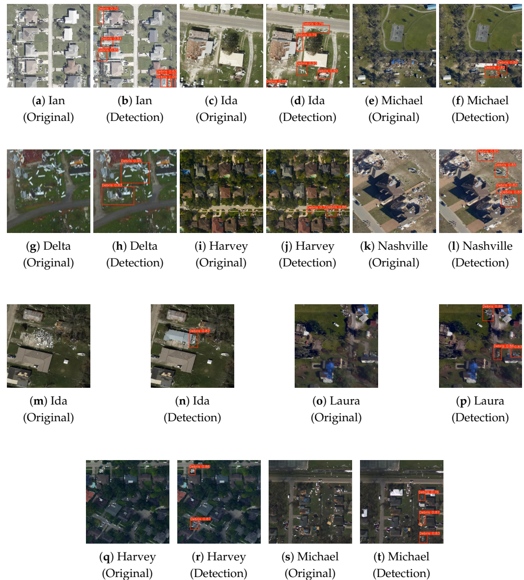
Figure 5. Representative original image tiles and YOLO-SDD detection results from multiple disaster-event groups, including hurricane and tornado scenes with residential, roadside, open-field, vegetation-covered, and structural-collapse conditions.
