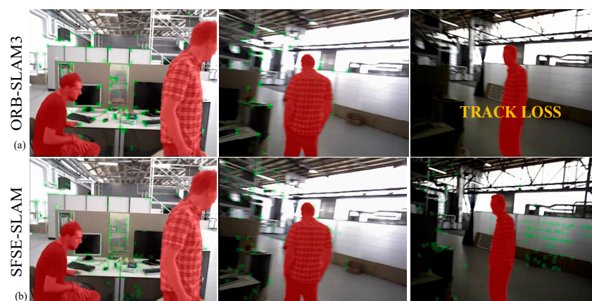
Figure 4. Comparative tracking performance on the Fr3-walking-rpy sequence: (a) ORB-SLAM3; (b) SFSE-SLAM.
