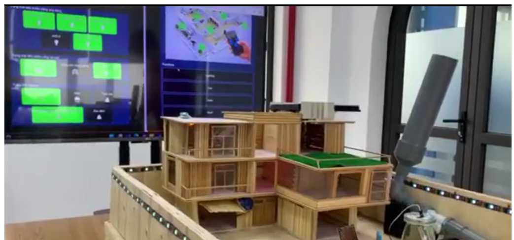
Figure 3. The laboratory smart home model used in the study; illustrating the process of operating smart home Internet of Things (IoT)-enabled monitoring control.
