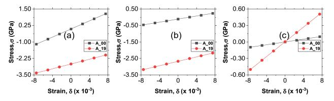
**Figure 6.** Calculated stress–strain curves for elastic stiffness constants (**a**)  $c_{11}$ , (**b**)  $c_{12}$ , and (**c**)  $c_{44}$  for samples A\_00 and A\_19.
