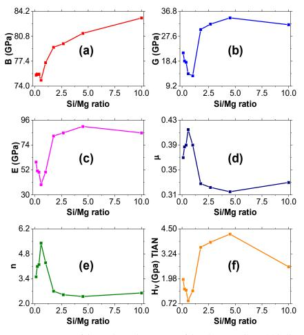
**Figure 7.** Variations of the mechanical properties of the Al–Mg–Si alloys: (**a**) bulk modulus, (**b**) shear modulus, (**c**) Young's modulus, (**d**) Poisson's ratio, (**e**) Pugh's ratio, and (**f**) Vickers hardness as a function of Si/Mg ratio.
