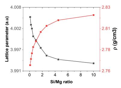
**Figure 5.** Graphs of equilibrium unit cell parameters and the densities of the alloy samples against the Si/Mg ratio.
