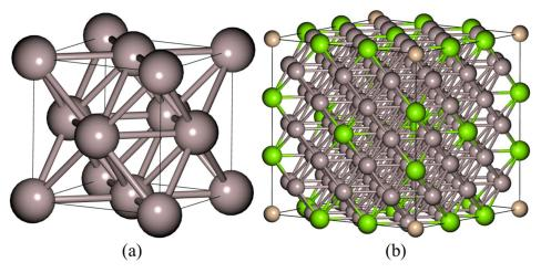
**Figure 1.** Three-dimensional structures of (**a**) an aluminium unit cell and (**b**) a supercell of the A\_19 (a  $3 \times 3 \times 3$  modeled Al–Mg–Si) alloy as visualized in Burai. The grey spheres represent the aluminium atoms; the brown spheres represent the silicon atoms; and the green spheres represent the magnesium atoms.
