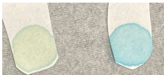
Figure 2. Bromocresol green sensor color change from green (acid) to blue (basic).
