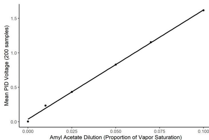
**Figure 2.** Calibration of Air Dilution Olfactometer. Figure shows the systematic change in the Photo Ionization Detector output as a function of systematic changes in the air dilution olfactometer ( $R^2 = 0.998$ ). X-axis shows the air dilution in effect on the olfactometer and Y-axis shows the change in sensor output.
