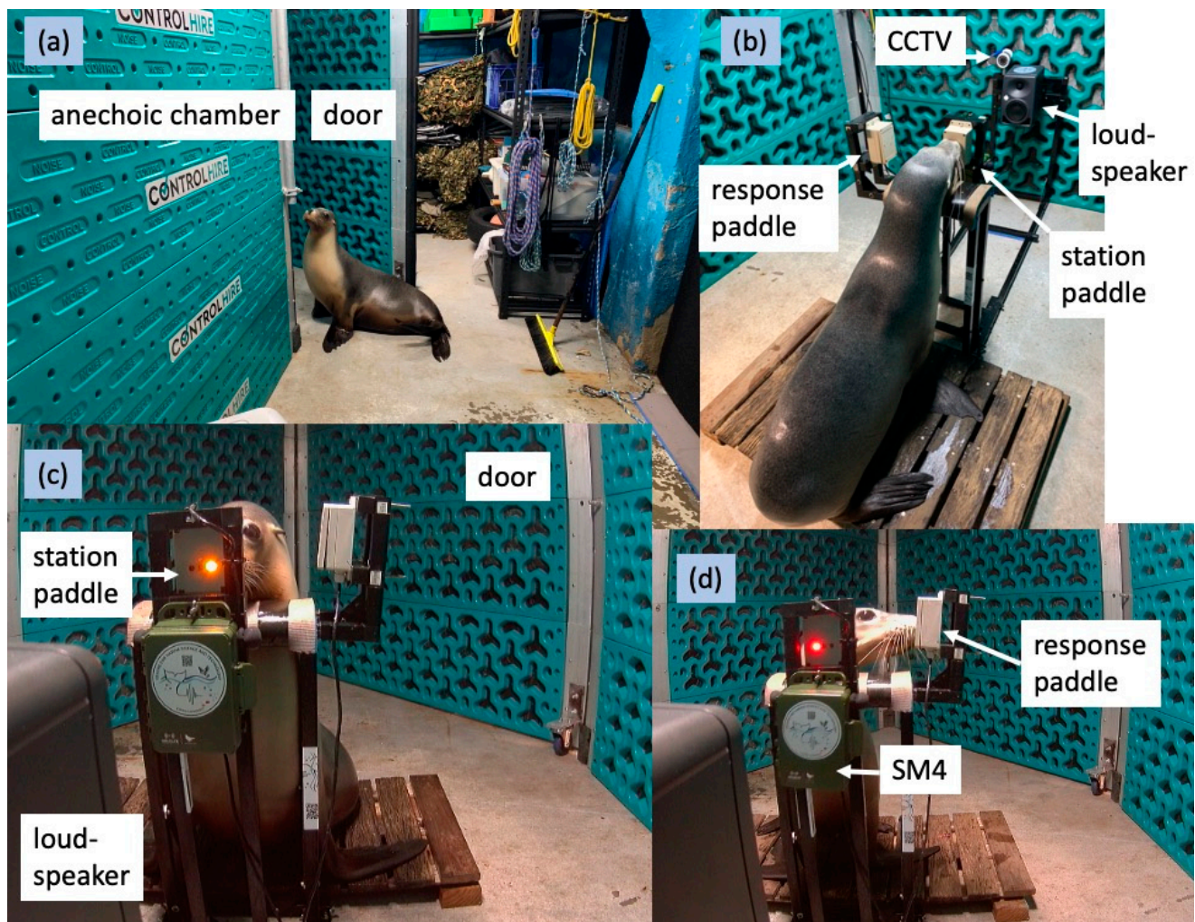
Figure 1. Photos of (a) Tarni walking into the anechoic chamber; (b) Nala stationing for a hearing test; (c) Tarni holding station, view from the CCTV, note the yellow diode indicating the animal is stationed properly; (d) Nala pressing the response paddle upon hearing a tone played from the loudspeaker in front of her, view from the CCTV, note the red diode indicating suppression of the response paddle.
