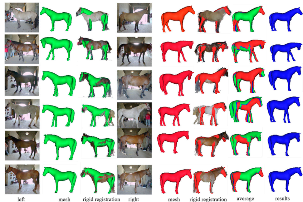
Figure 9. Representative results of left–right view mesh averaging and fusion. From left to right, the columns show the left-view RGB image, the corresponding single-view-reconstructed mesh (green), and its rigid registration with the acquired 3D point cloud, followed by the right-view RGB image, the corresponding single-view-reconstructed mesh (red), and its rigid registration result. The aligned left- and right-view-reconstructed meshes are subsequently averaged to generate the final fused mesh, shown in blue.
