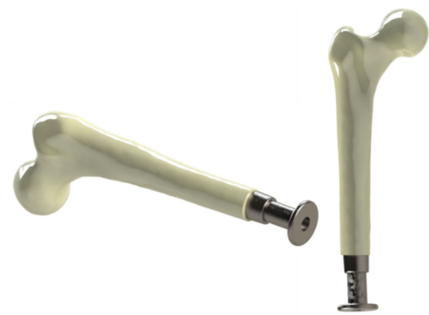
Figure 6. CAD model of assembly of bone and osseointegrated implants.
