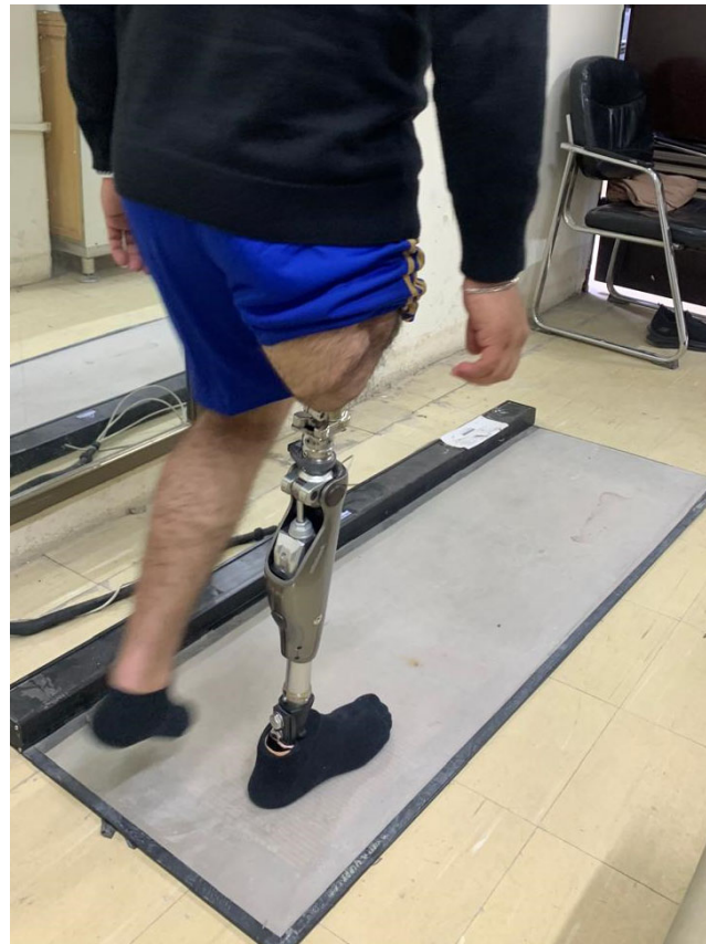
Figure 1. Instrumentation setup of the placement of the force plate for ground reaction force analysis.
