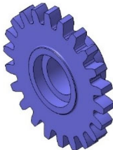
Figure 2. Conventional single-piece integrated steel gear.
