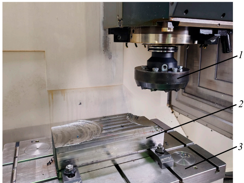
Figure 6. Cutting scheme: 1—cutting tool; 2—workpiece; 3—Kistler 9253B23 dynamometer.
