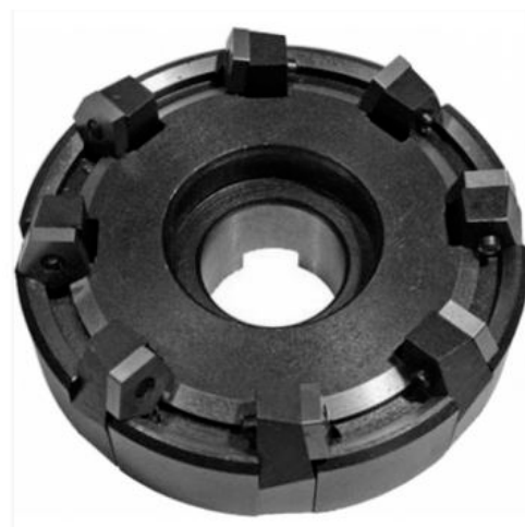
Figure 5. Face mill in accordance with GOST 26595-85. Adapted from [31].
