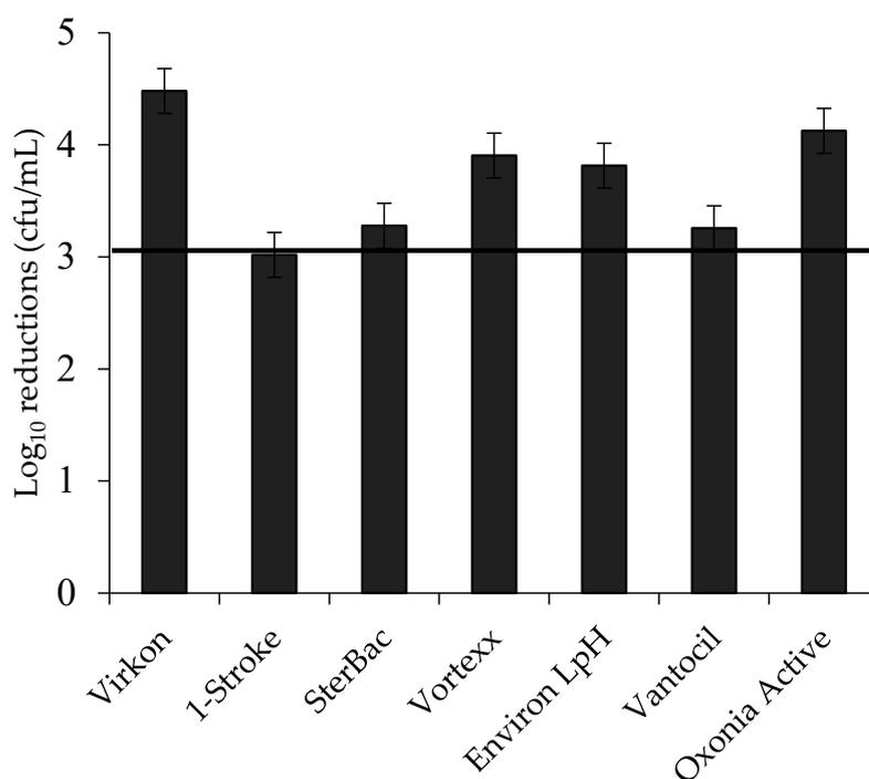
**Figure 7.** Log reductions in biofilm population densities ( $\log_{10}$  CFU/mL) for seven disinfectants. The means are averaged across the results for three food-borne pathogens on eight surfaces. The solid horizontal line shows the threshold for functional disinfection (3-log reduction). Error bars represent the standard error of the mean.
