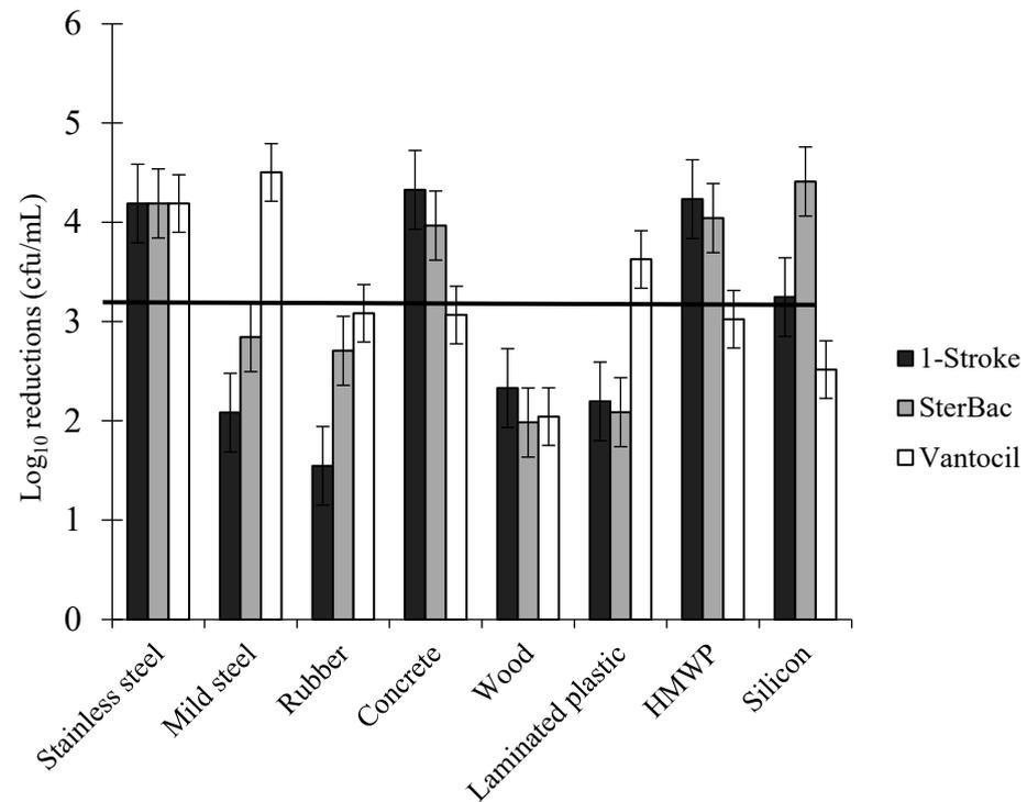
**Figure 9.** Log reductions in biofilm population densities (log<sub>10</sub> CFU/mL) for three disinfectants on eight surfaces. The means are averaged across the results for three food-borne pathogens. The solid horizontal line shows the threshold for functional disinfection (3-log reduction). Error bars represent the standard error of the mean.
