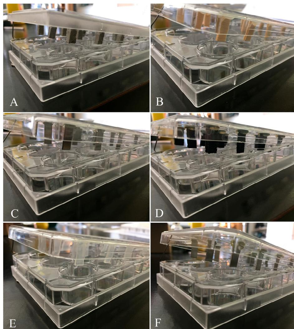
**Figure 1.** BEST™ Assay plates with coupons made from (A) concrete, (B) wood, (C) steel, (D) rubber, (E) UHMWP, (F) stainless steel.
