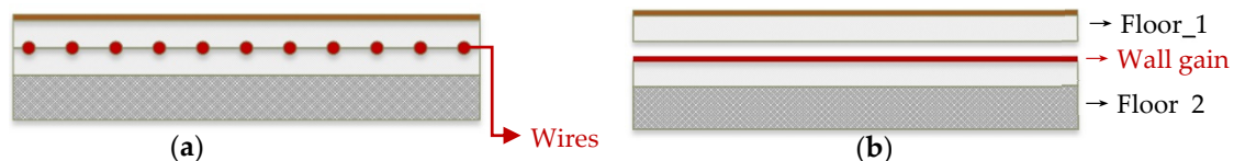
Figure 2. Conventional configuration of an EHF (electrically heated floors) (a); and configuration of the floor in TRNSYS with the added fictitious zone and the wall gain (b).
