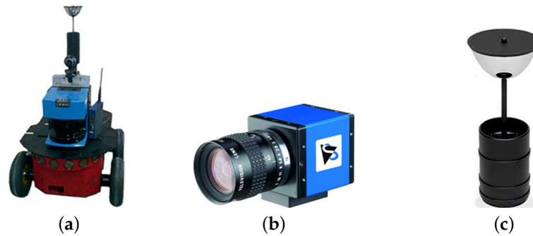
Figure 1. Real equipment: (a) Pioneer P3-AT with omnidirectional camera mounted, internal odometer and SICK-LMS200 laser range finder. Omron Adept Technology, Inc. 10 Columbia Drive, Amherst, NH 03031, USA; (b) CCD FireWire DMK21BF04. The Imaging Source Europe GmbH, Uberseeter 18, 28217 Bremen, Germany; (c) Eizho Wide 70 Mirror. Eizho Laboratory Ltd. Suminoue, Osaka, 559-0034, Japan.
