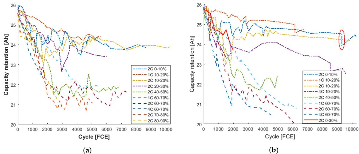
**Figure 2.** The ageing data used to parameterise the empirical ageing model in (a) 25 °C and (b) 35 °C. In (b), the data is also used to verify the model included. The vertical changes in capacity indicates stops in the testing due to maintenance, i.e., a rest period.
