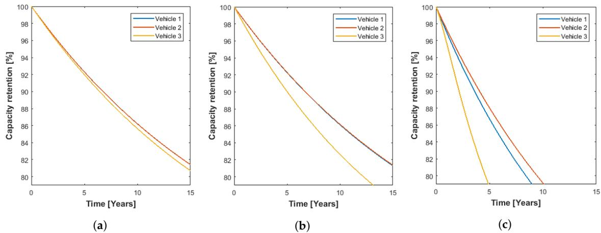
**Figure 9.** Ageing for the three vehicles while assuming driving according to, (a) WLTC medium; (b) WLTC; and (c) WLTC Extra High for five full charge/discharges per week all year around with a battery temperature of 30 °C.
