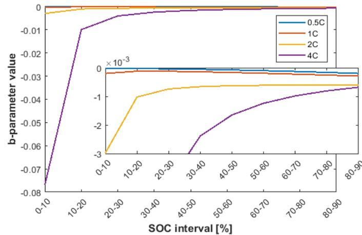
Figure 4. SOC and C-rate dependence for the *b* parameter in the ageing function.
