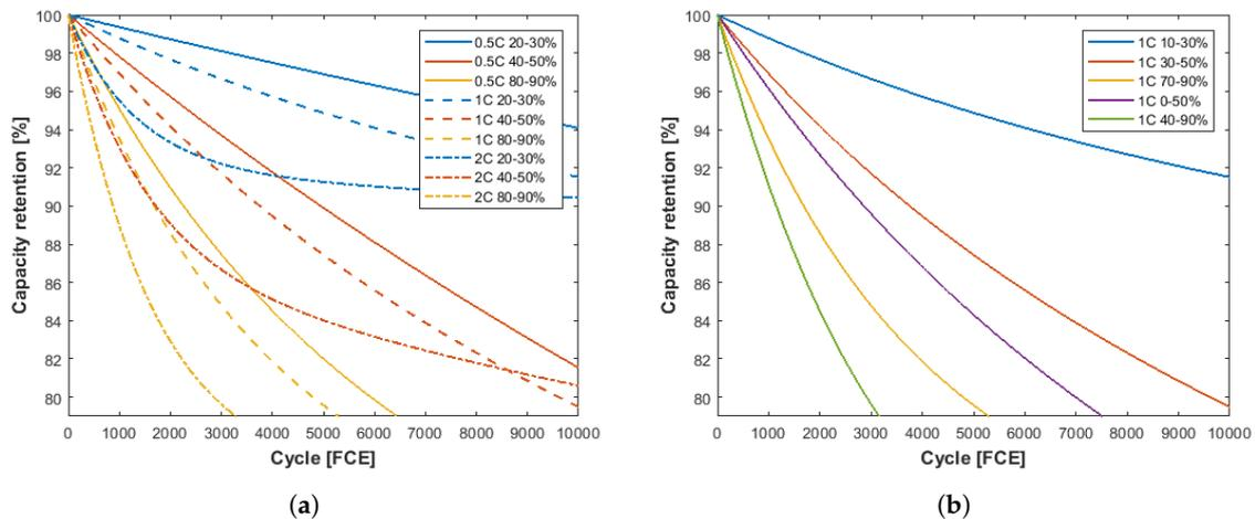
**Figure 8.** Model result at 30 °C starting at different SOC levels in (a) 10% Depth of Discharge (DOD) with 0.5C, 1C and 2C; and (b) 20% and 50% DOD with 1C.
