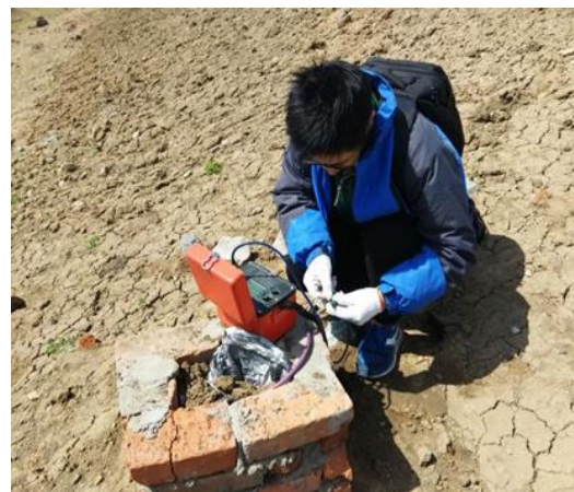
(b) Telescoping tube settlement gauge in field
