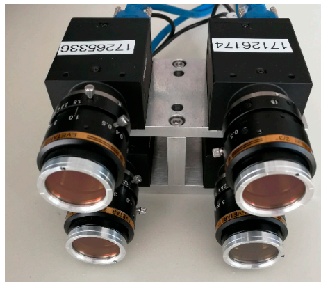
Figure 5. Real-time polarization dehazing imaging system.
