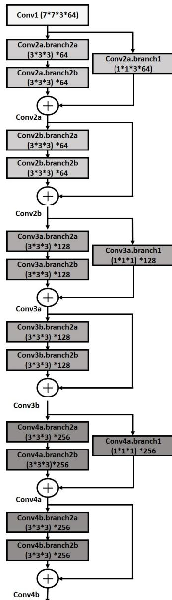
**Figure 3.** The four initial 3D residual blocks of Res3D.
