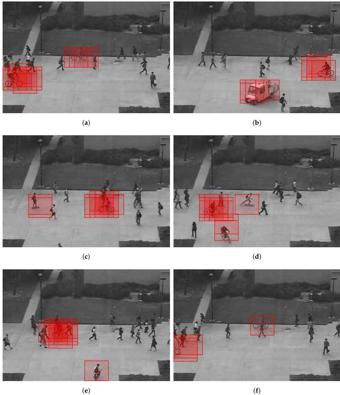
**Figure 7.** Detection of abnormal events in Ped2 Dataset. (a) Multiple bicycles detected; (b) Detection of multiple targets (bicycle and car); (c) Detection of multiple targets (bicycle and skater); (d) Detection of multiple targets (bicycles and skater); (e) Multiple bicycles detected; (f) Detection of multiple targets (bicycle partially obstructed and one wheel).
