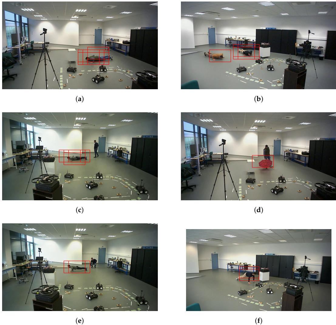
**Figure 6.** Detection of abnormal events. (a) Falling person; (b) Detection of multi-falling people; (c) Falling person in presence of walking one; (d) Detection of an object assumed as abnormal; (e) Falling person in presence of crouched person; (f) Falling person.
