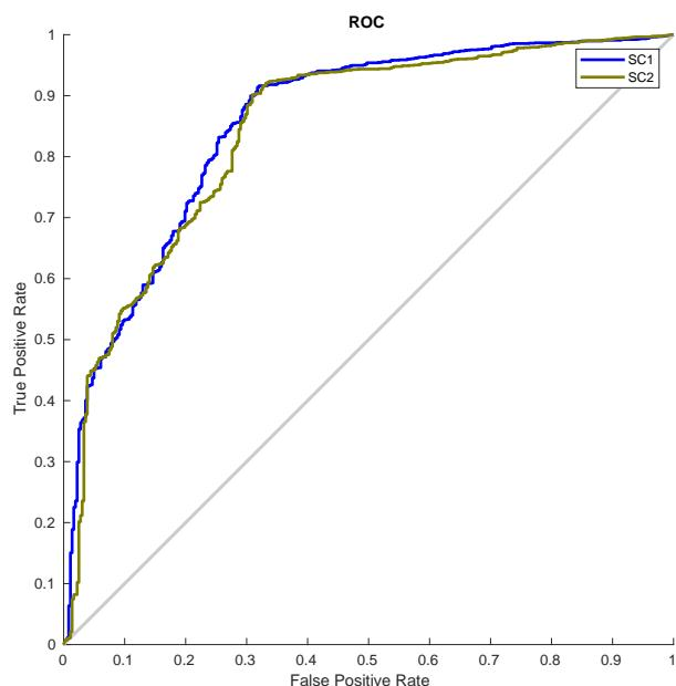
**Figure 8.** Receiver operating characteristic (ROC) curve of the proposed method. The blue and green curves are for the first and second scenarios, respectively. The Area Under the Curve (AUC) values for the two scenarios (SC1 and SC2) are 86% and 84%, respectively
