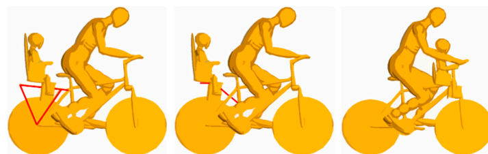
Figure 5. Mounting configurations of bicycle-mounted seat—rear-rack ( left ), rear-frame ( middle ), front ( right ).
