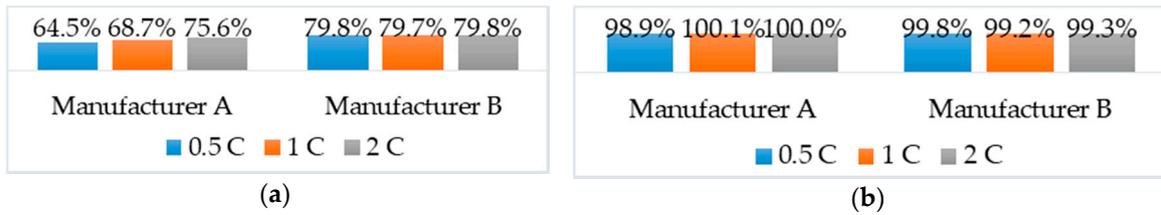
**Figure 15.** Effects of different charge rates on capacity of Ni-MH battery modules: (a) charge retention rate; (b) capacity recovery rate.
