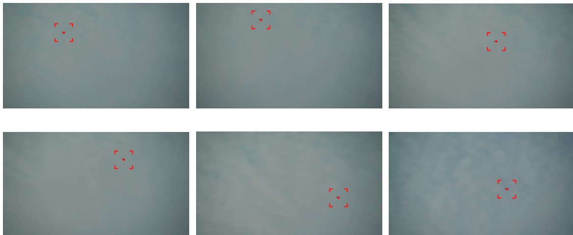
Figure 15. Results of the tracing test on cloudy days (drone flight altitude is 130 m).
