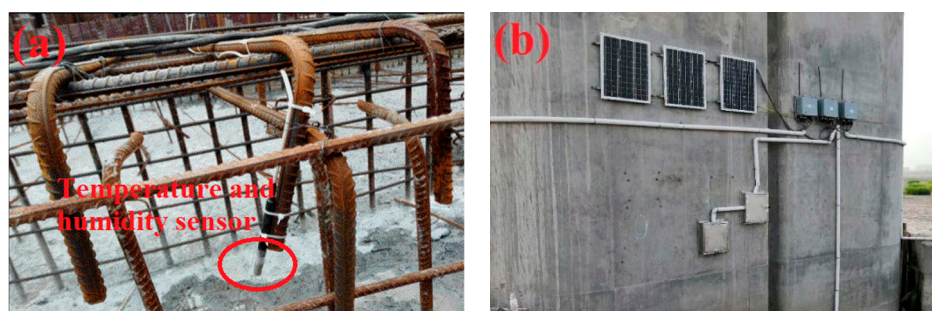
Figure 9. Sensor and apparatus. (a) Temperature and humidity sensor; (b) Wireless transportation apparatus (with solar panel).
